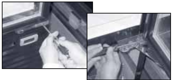
Adjusting door closing tension and leveling are simple processes with the Torque Master® feature. Using a flathead screwdriver, simply turn the screw on the front of the Torque Master to increase or decrease tension (left). Door leveling is accomplished by turning the screw on the side (right).
