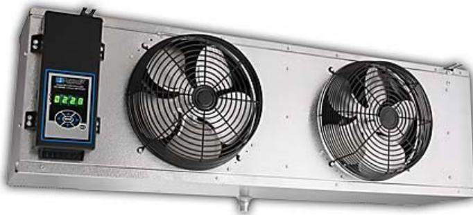
Many are familiar with the energy-saving qualities of the Master Controller Reverse Cycle Defrost option, but now there's a new way to expand on the savings. With the new evaporator fan cycling option, you can save an additional 2-4% more energy. The option saves electricity by cycling the evaporator fans during the compressor's off cycle. When the compressor is off, fan energy consumption is up to 60% less than if the fans were constantly running.
