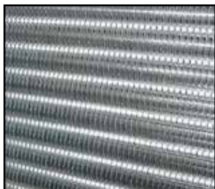
Close up of "fin style" condenser.
