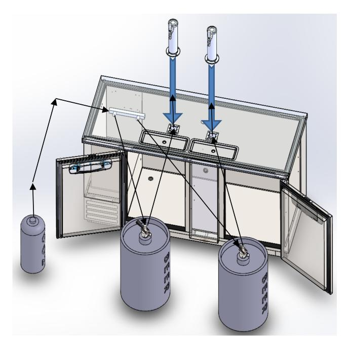
♦ Assemble Beer Line & CO<sub>2</sub> Line as above drawing.
