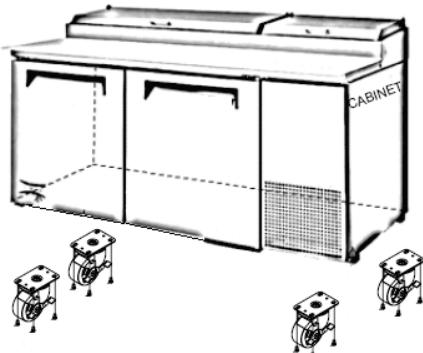
Note: Casters and bolts can be found packaged inside the cabinet. Install casters with brakes to the front of the prep table. The cabinet bottom has pre-punched holes for caster mounting. Install caster bolts tight to prevent future damage to cabinet base from loose casters.
