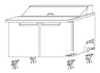
Once the Casters or Legs installed the unit can be returned to its upright position. Be sure to work in pairs when returning the unit to the upright position.
