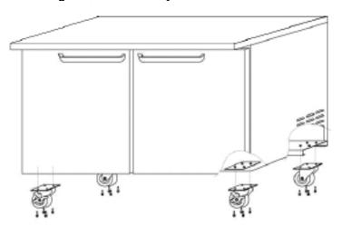
Once the Casters or Legs are installed the unit can be returned to its upright position. Be sure to work in pairs when returning the unit to the upright position.
