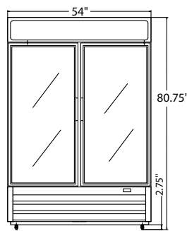
MBRGM48HB/MBFGM48HB ELEVATION VIEW
