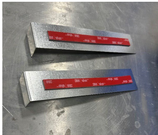
Figure 26 – End Skirt Brackets
